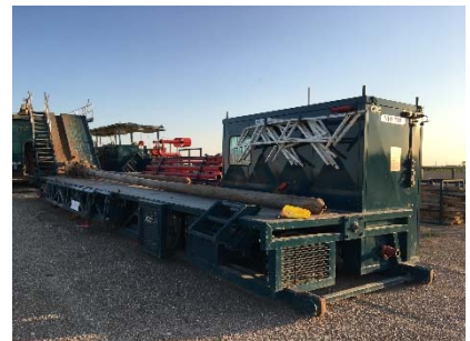
3.8 Catwalk and Manifold Shack
