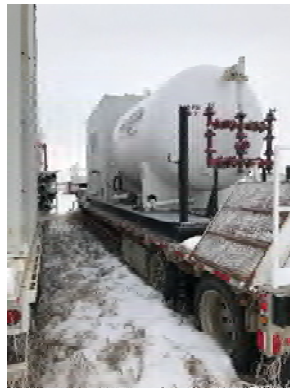
PT261: 2000 Micoda Process P-Tank trailer, 200 psi, 14m 3
