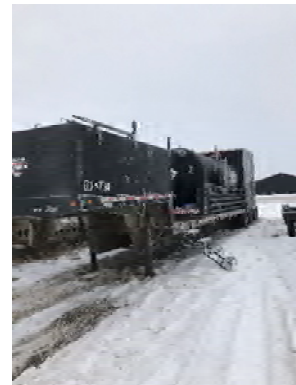
PT 256: 2006 Silverado Oilfield P-Tank trailer, 250 psi, 14m 3
