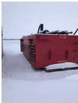
Flow Back Tank
