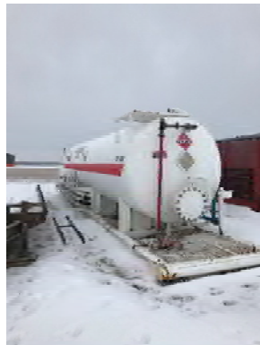
PT 255: 1953 Adams Welding P-Tank, 100 psi, 33m 3
