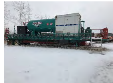
PT 256: 2006 Silverado Oilfield P-Tank trailer, 250 psi, 14m 3
