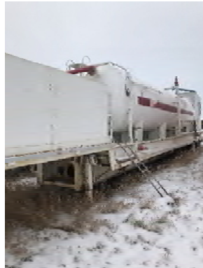
PT 252: 1953 Adams Welding P-Tank trailer, 100 psi, 33m 3
