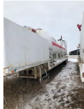
PT 253: 1953 Adams Welding P-Tank trailer, 100 psi, 33m 3
