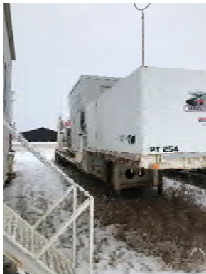
PT 254: 1998 BWS Man F. P-Tank trailer, 250 psi, 18m 3
