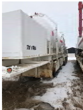
PT 258: 1953 Adams Welding P-Tank trailer, 100 psi, 33m 3
