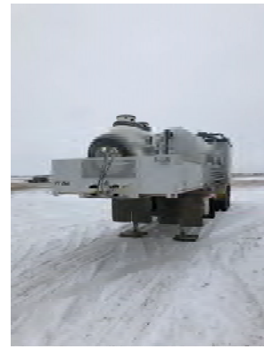
PT 262: 2001 Micoda Process P-Tank trailer, 250 psi, 18m 3
