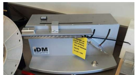
Stiffness of Cloth Tester - Drapability
