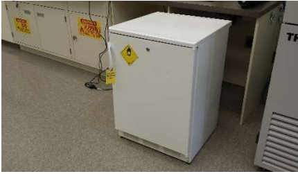
#80 Refrigerator Flammable Safe
